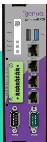
The Industrial Firewall genuwall from the German manufacturer genua offers four firewall ports to enable zone creation.
