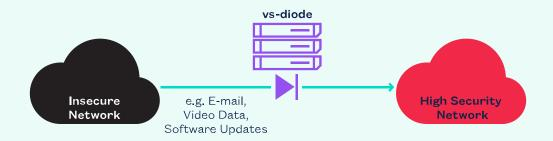
Transfer from black to red network via vs-diode
